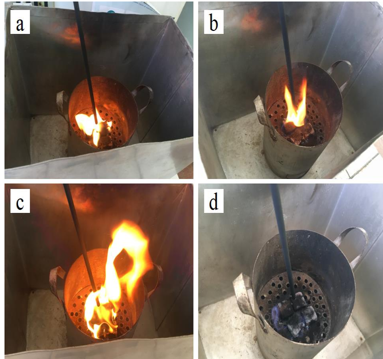
Fig. 14 Fire stages during the combustion of the particleboards; a) 1 min; b) 3 min; c) 5 min; d) 10 min
