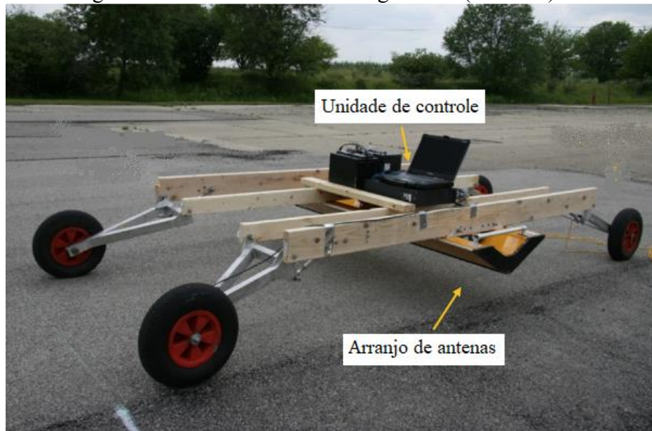
Figura 10 - "3D Ground Penetrating Radar" (GPR 3D)
