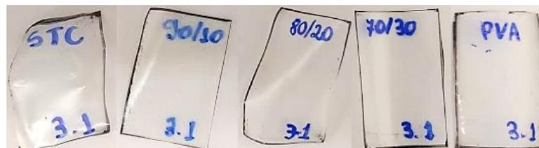
Fig. 1. Photo of the developed films, already cut for isothermal/diffusion analysis (from left to right): MSTC, 90S10P, 80S20P, 70S30P, and PVOH.
