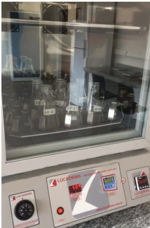
Figura 3.2 – Incubadora shaker com as amostras
